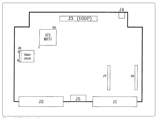
Figure 4.3 Positions of connectors
